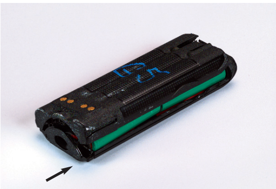
Multiplier M8923HX Battery Drop Test Failure, Splitting along right side
