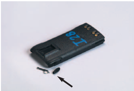
Honeywell H9013 Vibration Test Failure, Latches Damaged
